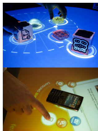
Figure 1. Hybrid surfaces such as ReacTable and Microsoft Surface allow users to directly manipulate digital objects using multi-touch input. Physical objects are also recognized and have effects in the digital world.
